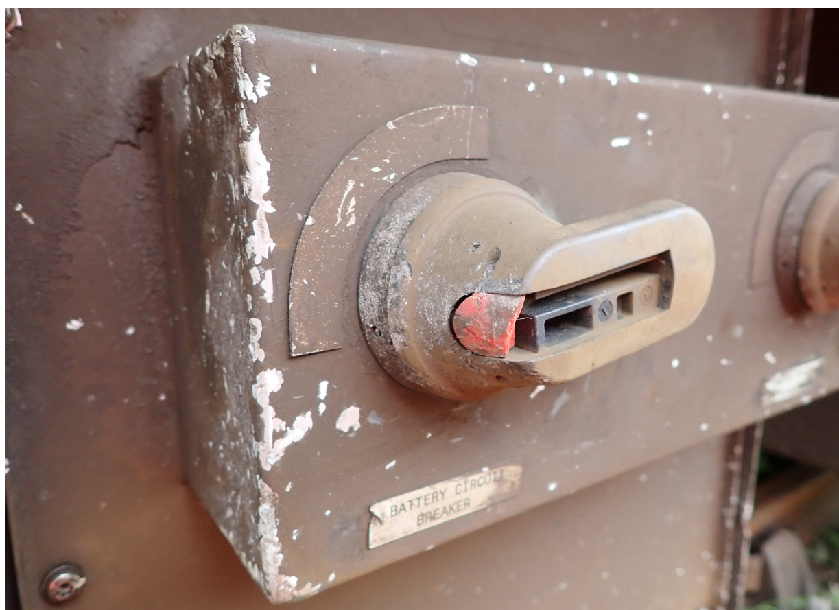
Figure 17: Damage caused to the battery isolation switch as it was knocked to the isolated position during the derailment.
