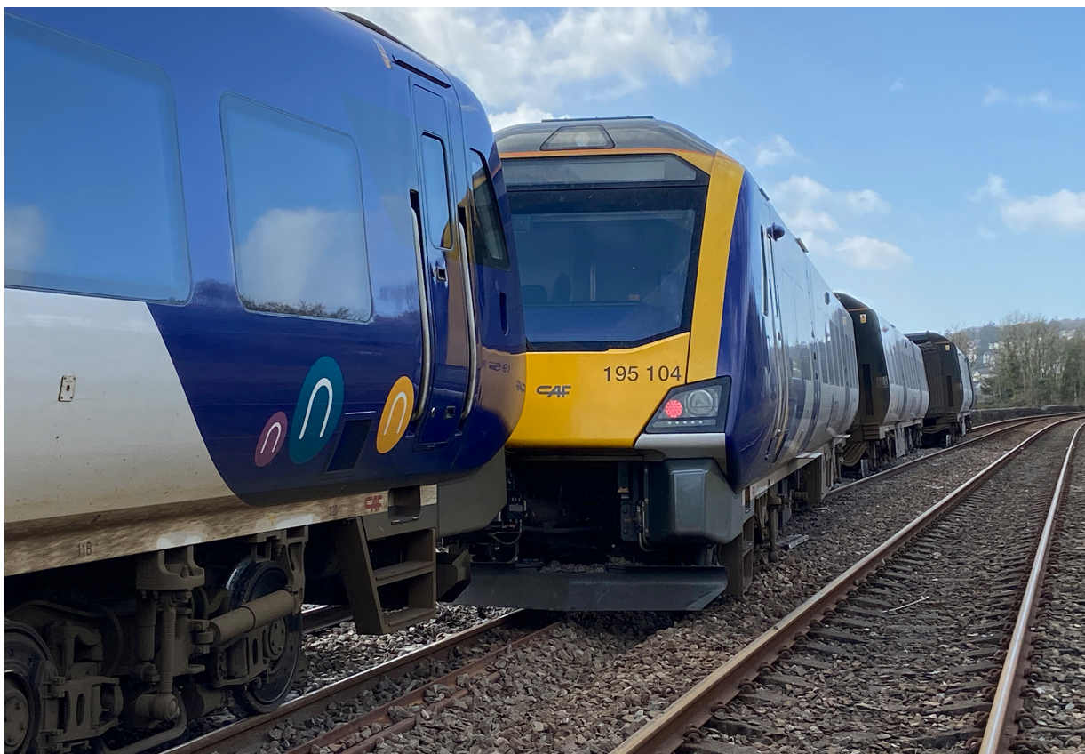
Figure 4: Train 2C37 following the derailment.
