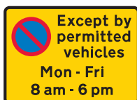
Repeater sign within a loading area
