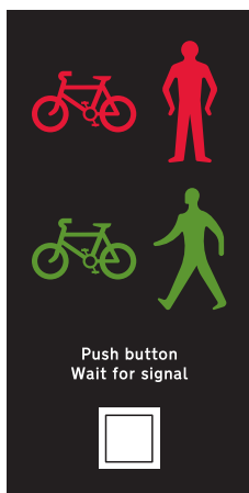
Near-side signals for toucan crossing
